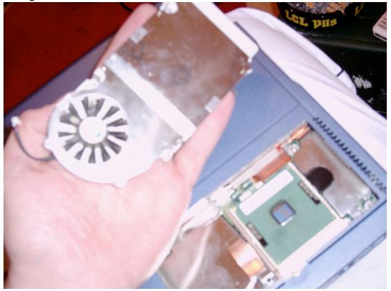
Next remove the keyboard, there are three little clips at the bottom of the keyboard, there sprung clips, so just push a small knife in there and they'll just pop right out, Easy. There is a little ribbon under there, just remove this and the silver heat plate under that.
