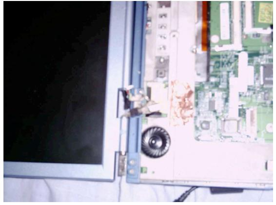
Now, remove all the screws under the base unit, there is one hiding under the battery too. Then pull out the DVD-ROM drive and then the whole machine "should" lift out the outer casing, be sure to look for more screws that you may have missed out. They are some securing mounts on the ports at the back of the unit, remove these with a small spanner or pointed nosed pliers like I did.
