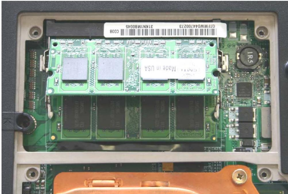
**Illustration 6 – Insert memory module at 45-degree angle**
