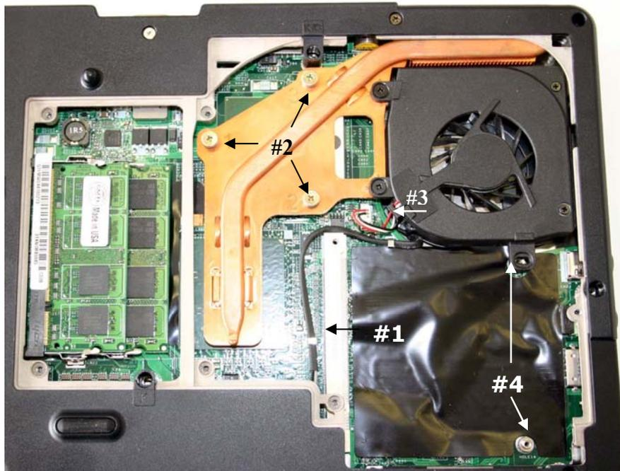
**Illustration 5 – CPU, Thermal Assembly, and Discrete Graphics**
